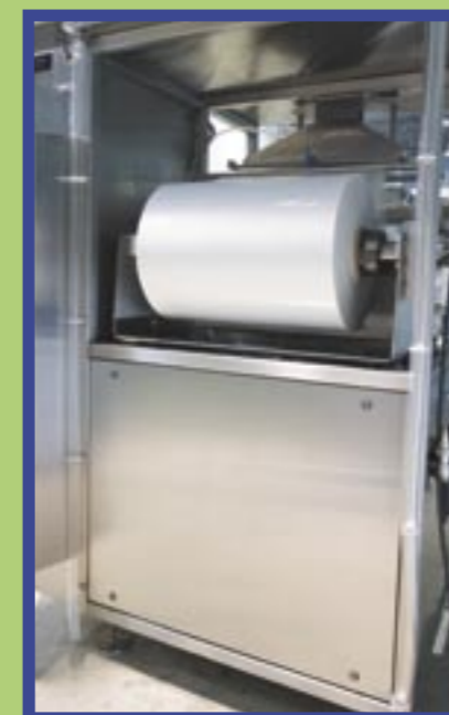
Roll stock integrated into machine chassis requiring less floor space.
