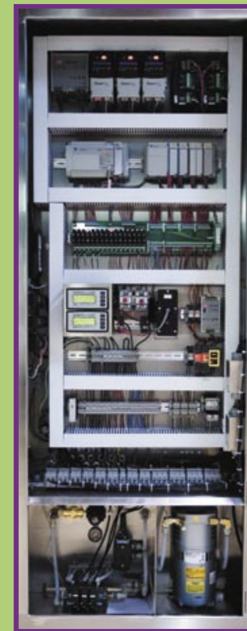
All electrical/pneumatic components housed in a stainless steel panel.
